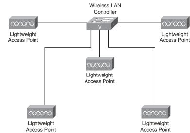
Figure 2-7 Cisco Wireless Switched Network
