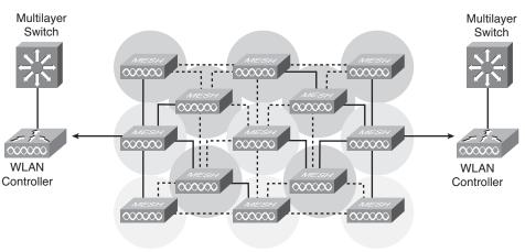
Figure 2-8 Cisco Wireless Mesh Network Architecture
